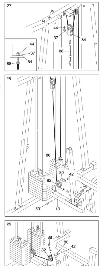
29. Wrap the Press Cable (88) around a 3 1/2" Pulley (82). Attach the Pulley and a Cable Trap (80) to the other bracket on the Press Base (13) with a 3/8" x 2" Bolt (50) and a 3/8" Nylon Locknut (42). Make sure the Cable Trap is turned to hold the Cable in place.
